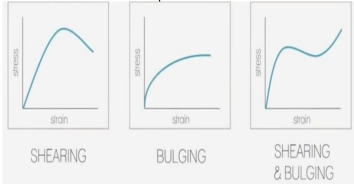
Types of failure & their corresponding stress-strain plot
