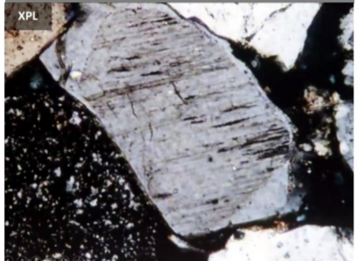
Feldspar core with weathering product along cleavage plane, & dust line divided the core from overgrowth
