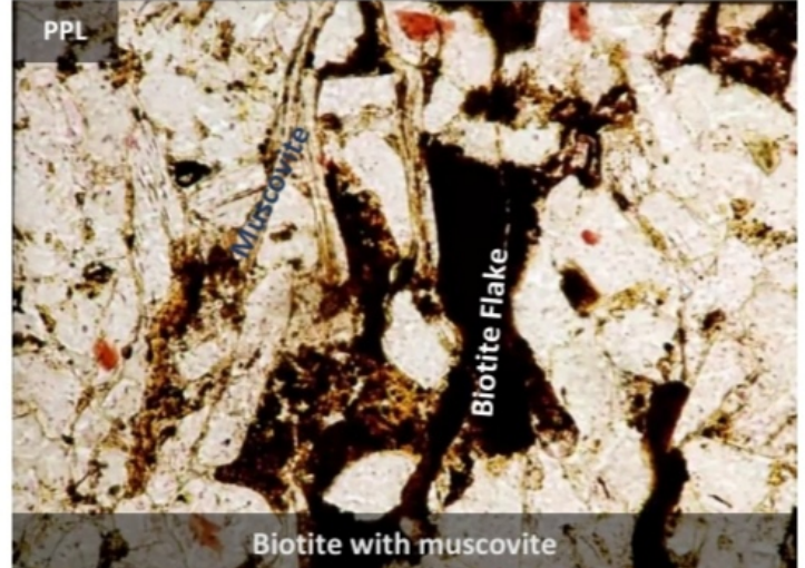
Biotite swelling during weathering & Diagenesis & altered into clay minerals such as Kaolonite
