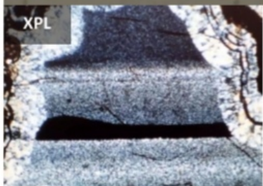
(Right) cryptocrystalline quartz surrounded by chalcedony, (Left) chalcedony: variety characterized by Zebra-extinction
