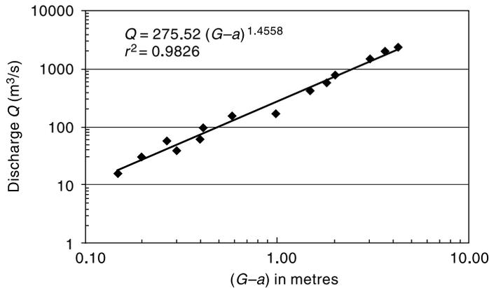
Fig. 4.24(b) Stage-discharge Relationship (Logarithmic Plot) – Example 4.4
