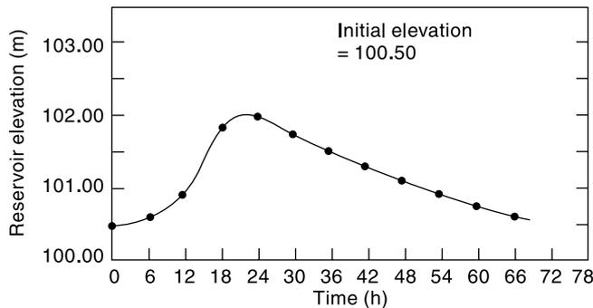
Fig. 8.4 Variation of reservoir elevation with time – Example 8.1
