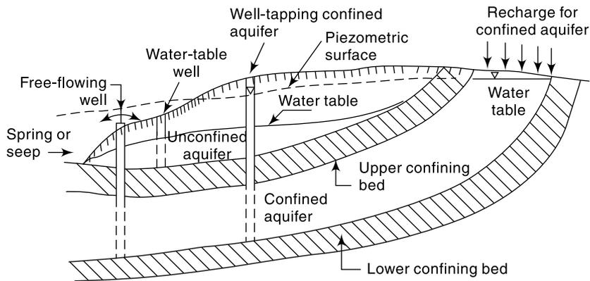
Fig. 9.2 Confined and Unconfined Aquifers
