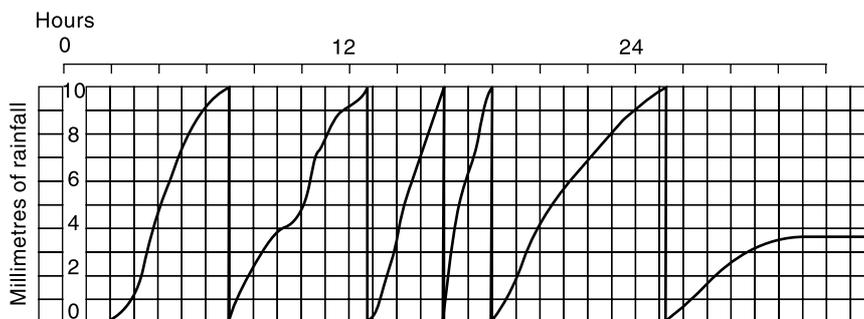
**Fig. 2.6** Recording from a Natural Syphon-type Gauge (Schematic)
