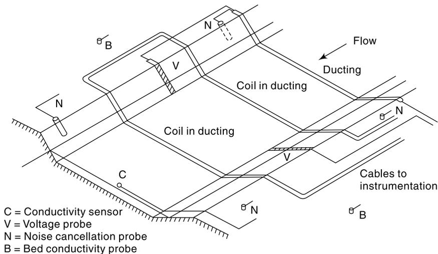
Fig. 4.18 Electromagnetic Method
