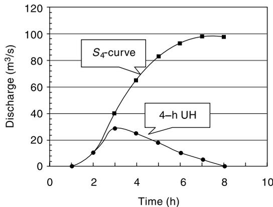
Fig. 6.17 Construction of  $S_4$ -curve – (Example 6.10)
