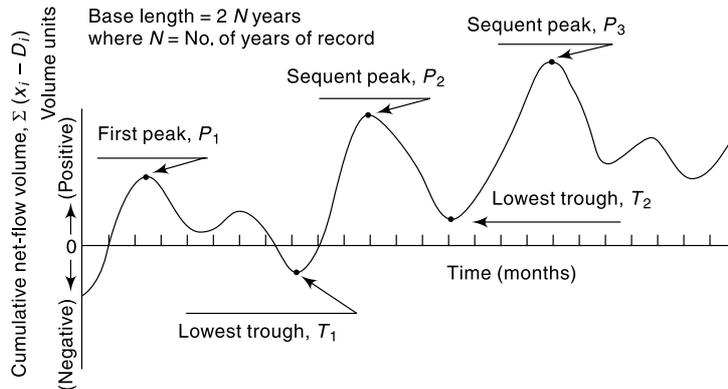
**Fig. 5.15** Residual Mass Curve – Definition Sketch for Sequent Peak Algorithm
