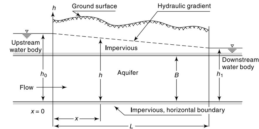
Fig. 9.8 Confined Groundwater Flow between Two Water Bodies
