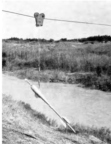
**Fig. 4.12(b)** Neyrtec Type Meter in a Cableway
