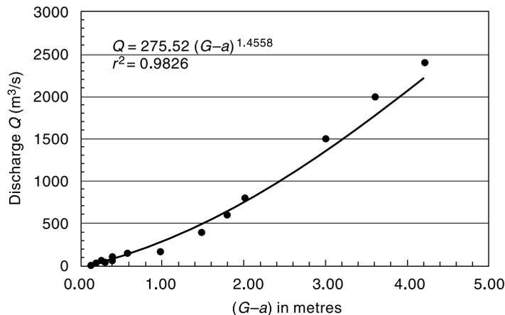
Fig. 4.24(a) Stage-discharge Relation (Arithmetic Plot) – Example 4.4
