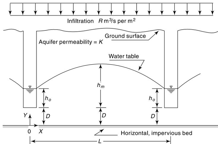
Fig. 9.24 Seepage to open ditches – Problem 9.10
