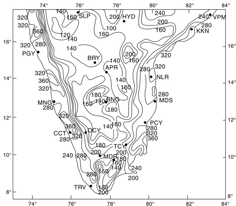
**Fig. 2.21** Isopluvial Map of 50 yr-24 h Maximum Rainfall (mm)
