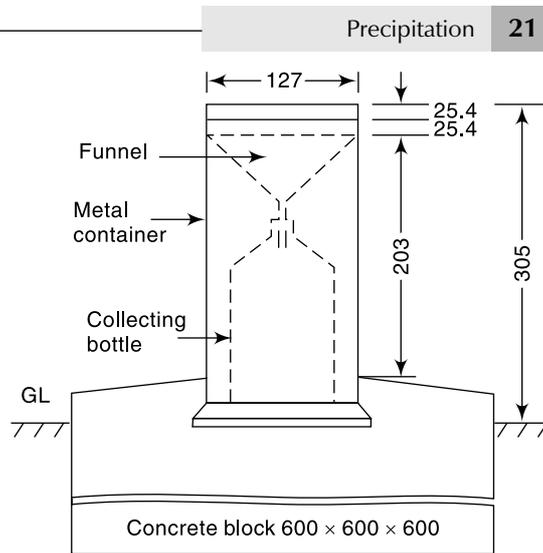
**Fig. 2.5** Nonrecording Raingauge (*Symons' Gauge*)
