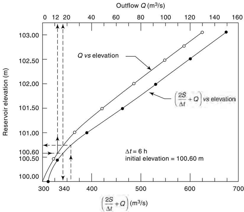
Fig. 8.5 Goodrich method of storage routing—Example 8.2
