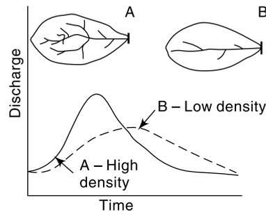
**Fig. 6.3** Role of Drainage Density on the Hydrograph
