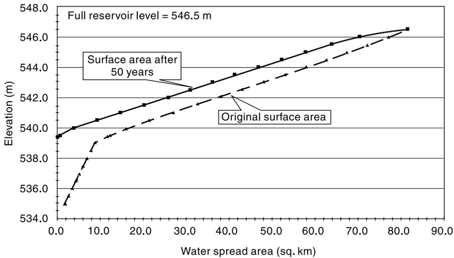
Fig. 10.7(a) Reservoir Elevation - Area Curves—Example 10.6
