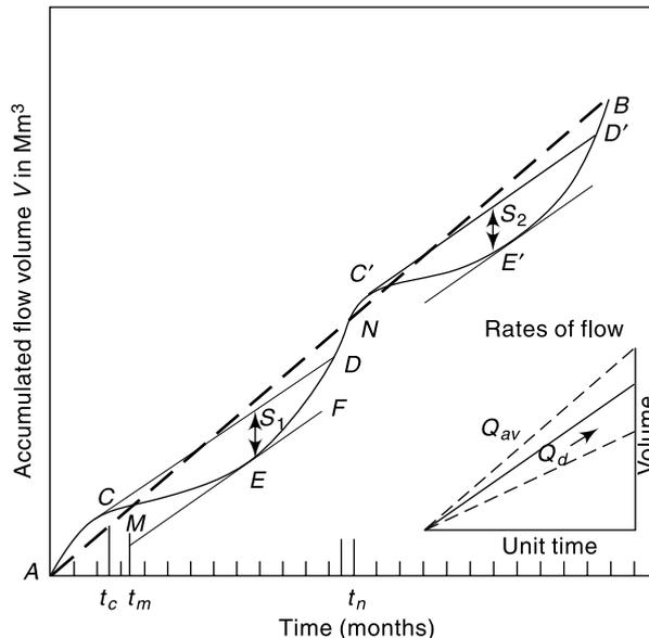
Fig. 5.11 Flow-Mass Curve
