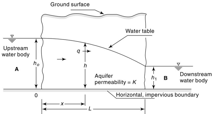
**Fig. 9.11** One Dimensional Unconfined Flow without Recharge
