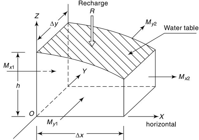
**Fig. 9.9(b)** Definition Sketch - Unconfined flow with Recharge
