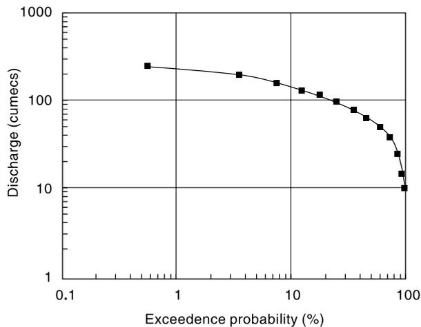
Fig. 10.2 Flow Duration Curve – Example 10.1
