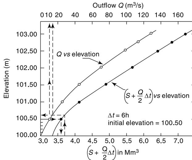
Fig. 8.2 Modified Pul's method of storage routing
