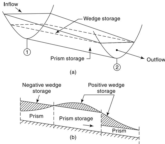
Fig. 8.7 Storage in a channel reach
