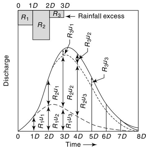
**Fig. 6.14** Unit hydrograph from a Complex Storm
