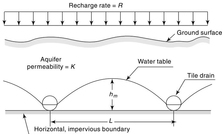
**Fig. 9.12** Tile Drains under a Constant Recharge Rate
