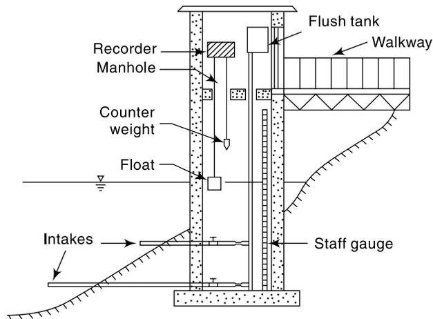
Fig. 4.2 Stilling well Installation
