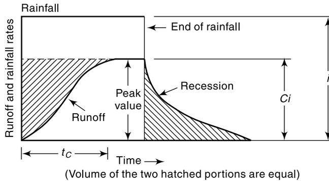
**Fig. 7.1** Runoff Hydrograph due to Uniform Rainfall
