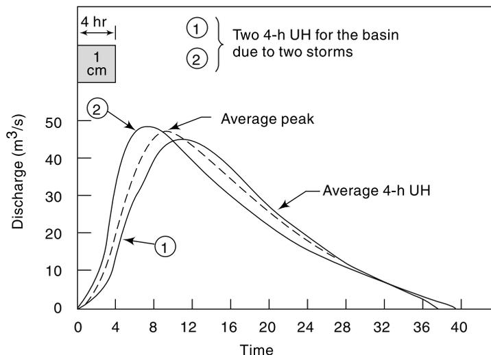
Fig. 6.12 Derivation of an Average Unit Hydrograph
