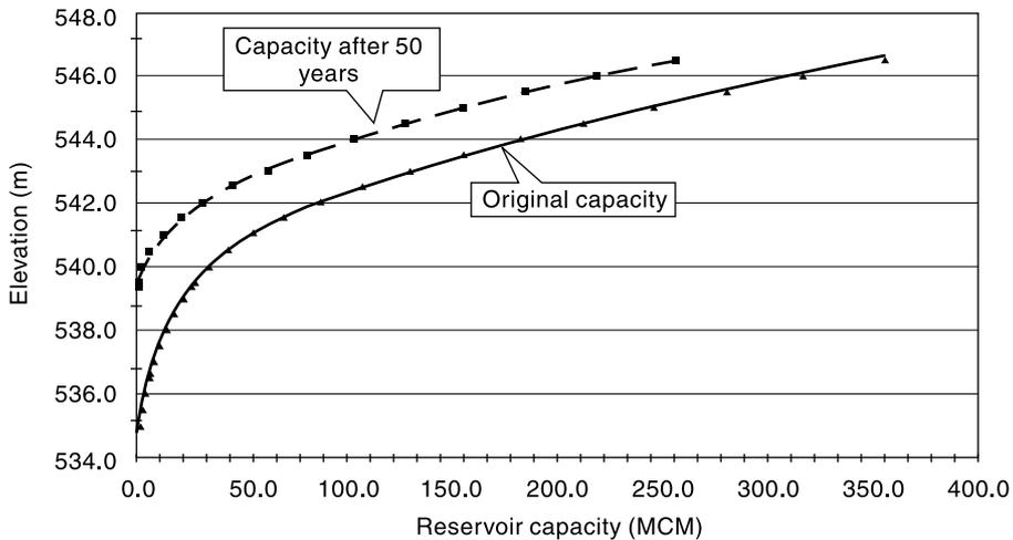
Fig. 10.7(b) Reservoir Elevation - Capacity Curves—Example 10.6
