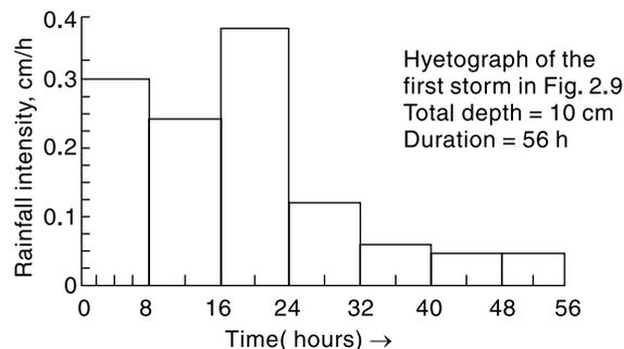
Fig. 2.10 Hyetograph of a Storm
