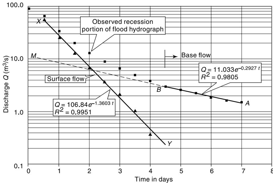
Fig. 6.4 Storage Recession Curve – Example 6.1
