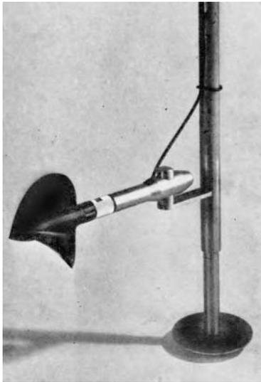
**Fig. 4.12(a)** Neyrtec Type Current Meter for use in Wading
