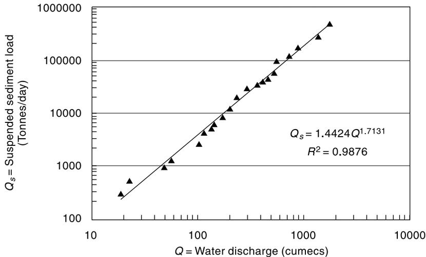
Fig. 10.1 Sediment rating curve (Schematic)
