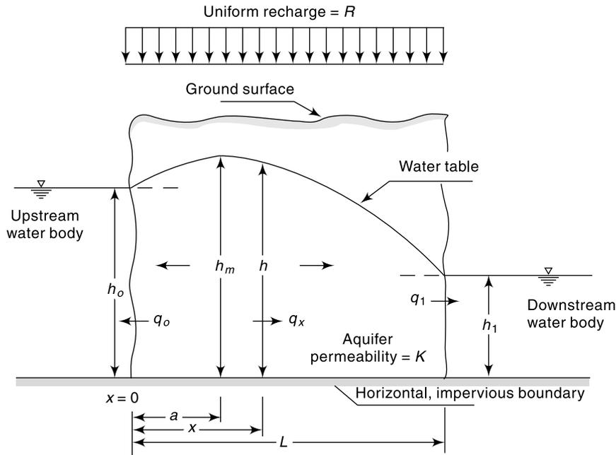
Fig. 9.10 One Dimensional Dupuit Flow with Recharge
