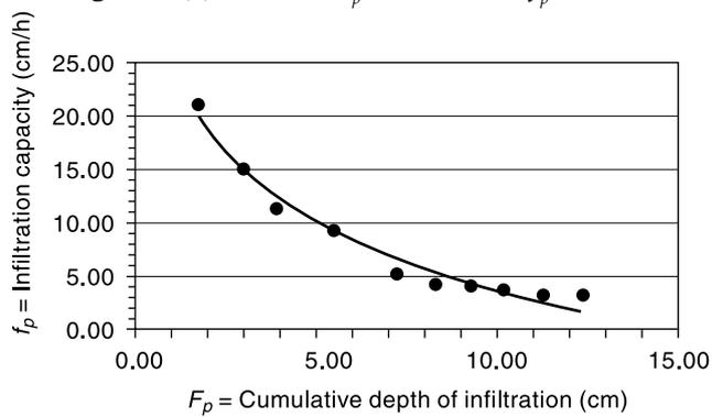
Fig. 3.14 (b) Plot of  $f_p$  vs  $F_p$
