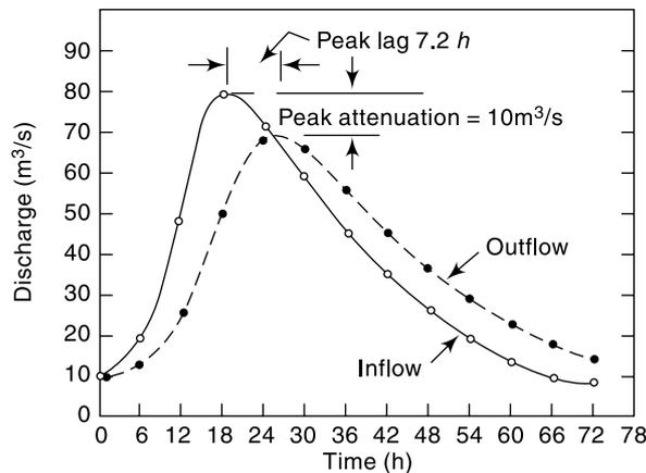
**Fig. 8.3** Variation of inflow and outflow discharges—Example 8.1
