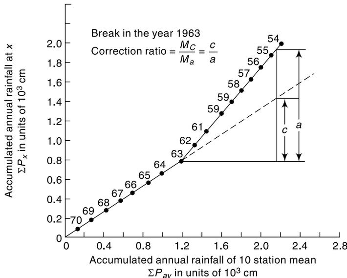
Fig. 2.7 Double-mass Curve
