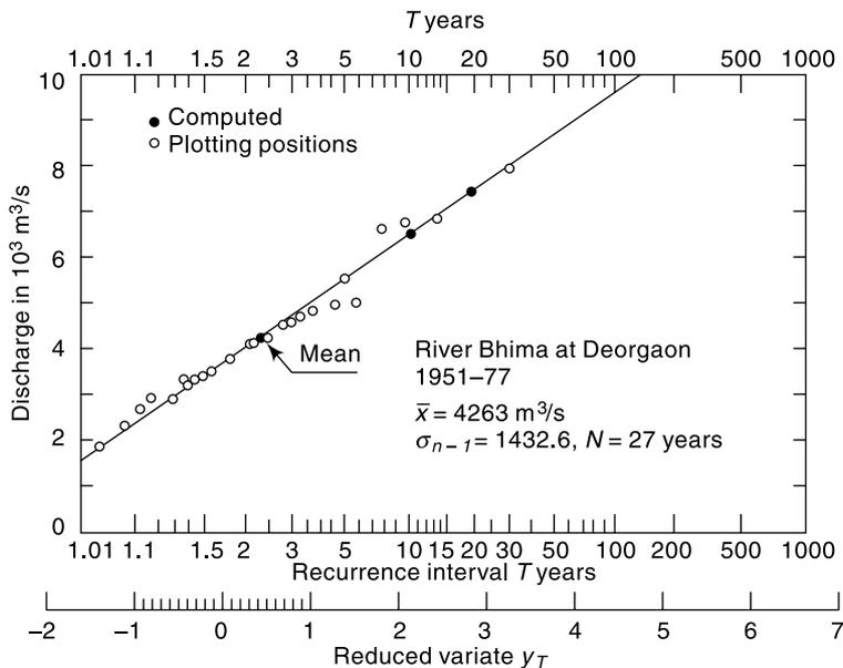
Fig. 7.3 Flood probability analysis by Gumbel's Distribution
