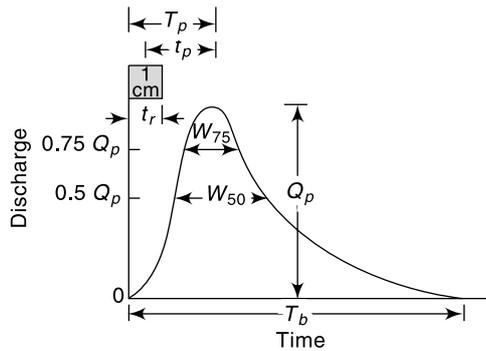
Fig. 6.20 Elements of a Synthetic Unit Hydrograph
