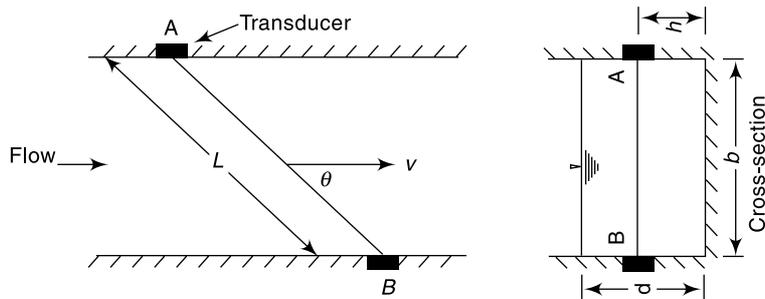
Fig. 4.19 Ultrasonic Method
