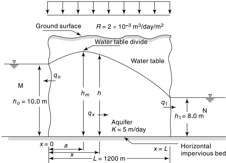
Fig. 9.14 Schematic Layout—Example 9.5
