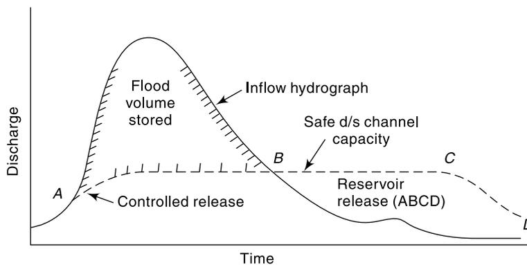
**Fig. 8.15** Flood control operation of a reservoir
