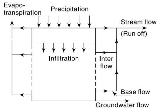
Fig. 1.2 Transportation Components of the Hydrologic Cycle
