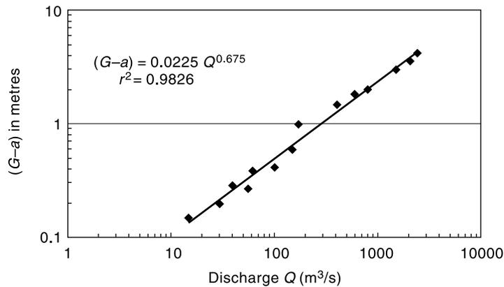
Fig. 4.29(a) Discharge-stage Relationship: Example 4.6 (Logarithmic Plot)
