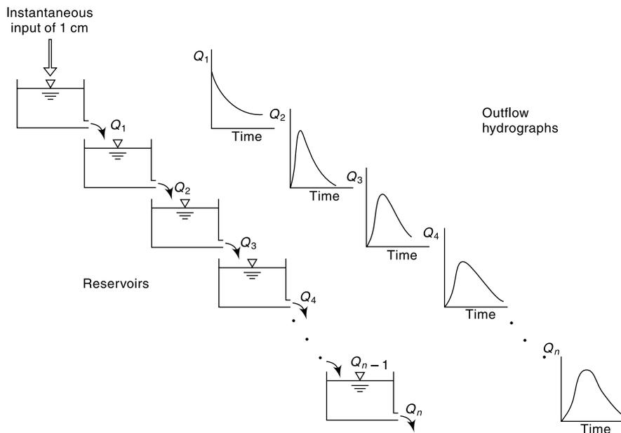
Fig. 8.13 Nash Model: Cascade of Linear Reservoirs
