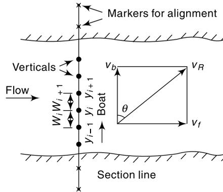
Fig. 4.15 Moving-boat Method
