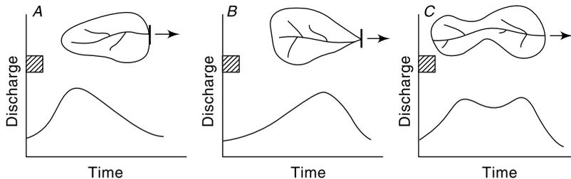
**Fig. 6.2** Effect of Catchment Shape on the Hydrograph
