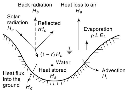
Fig. 3.4 Energy Balance in a Water Body
