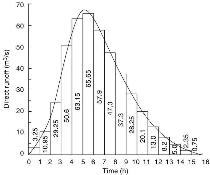
Fig. 8.14(b) Direct runoff hydrograph of Example 8.7
