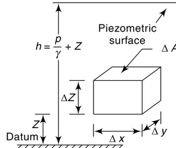
Fig. 9.7 Volume element of a compressible aquifer
