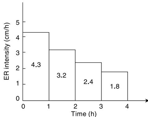
**Fig. 8.14(a)** Excess rainfall hyetograph of Example 8.7
