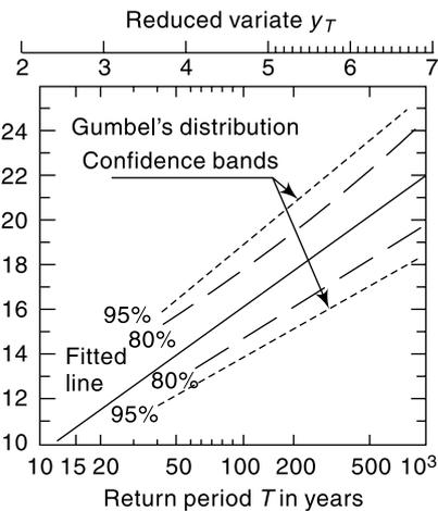
**Fig. 7.4** Confidence Bands for Gumbel's Distribution— Example 7.7
