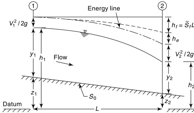
Fig. 4.21 Slope-area Method
