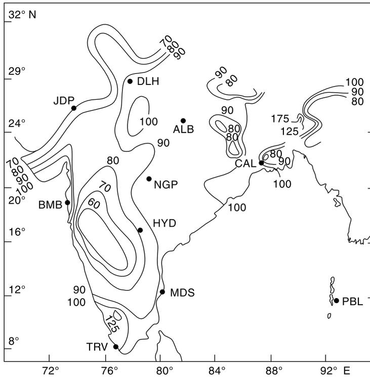
**Fig. 2.22** Isopluvial Map of 50 yr-1 h Maximum Rainfall (mm)
