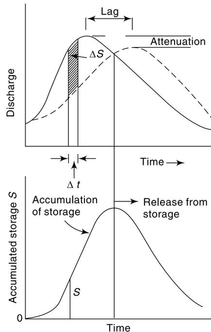
Fig. 8.8 Hydrographs and storage in channel routing
