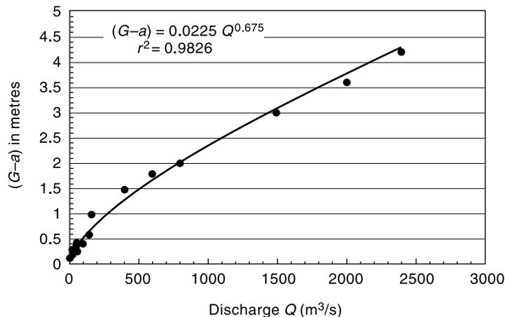
Fig. 4.29(b) Discharge-stage Relationship: Example 4.6 (Arithmetic Plot)
