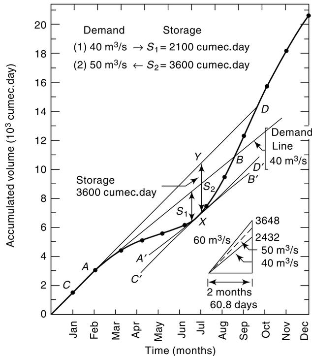
Fig. 5.12 Flow-Mass Curve—Example 5.9
