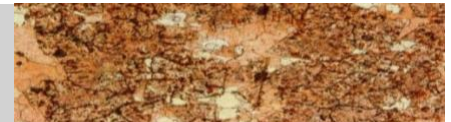
Dedolomite with spar rhombs outlined by Fe-oxide & inclusion indicative of former dolomite rhombs
